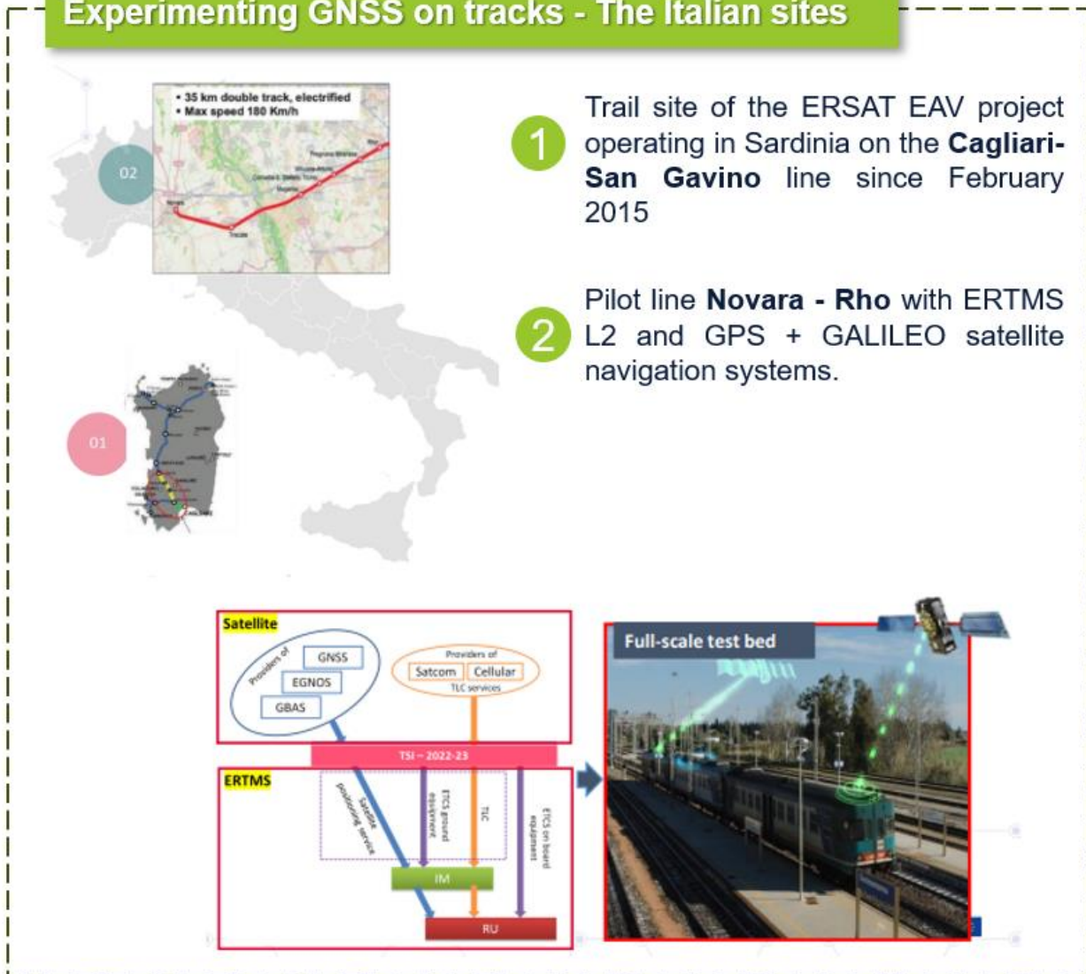
Figure 4: Scheme of GNSS experimenting on tracks
