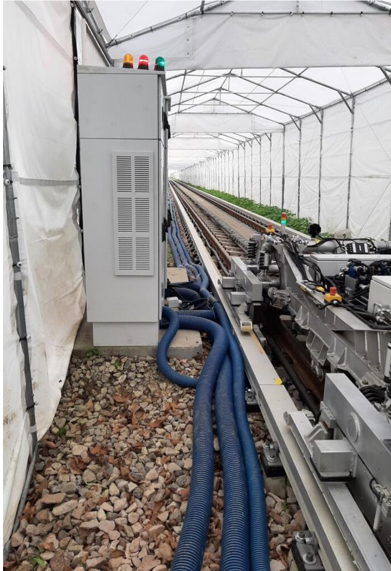
Figure 10: The segment switch and cabling in Nevomo test facility in Nowa Sarzyna
