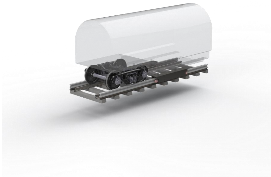
Figure 33 - Ironlev hybrid system with EMS lateral guidance – overview (Source: Ironbox)
