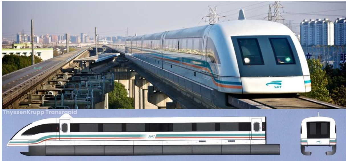
Figure 7 - Outline (above) and picture (below) of the Transrapid SMT (Shanghai Maglev Transportation Development) vehicle
