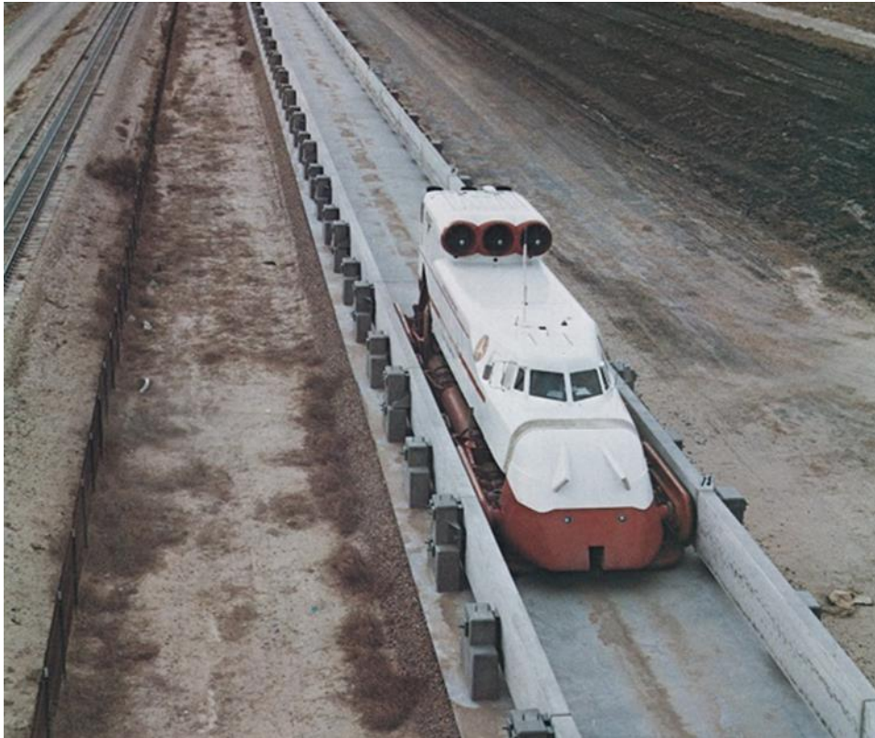
Figure 8 - Grumman Aerospace Corporation started design of their Tracked Levitated Research Vehicle (TLRV) in March 1970
