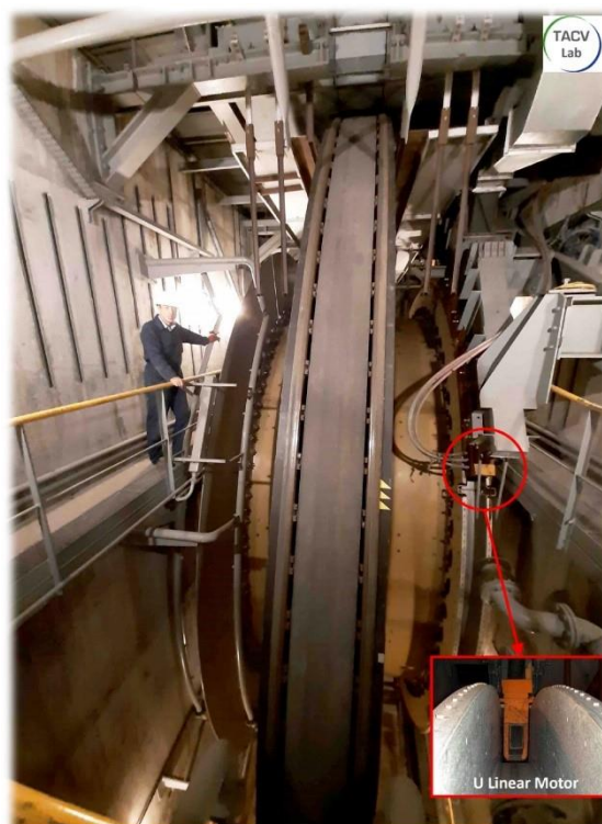
TACV Lab. Grenoble Wheel Laboratory, 13m diameter, 300km/h
