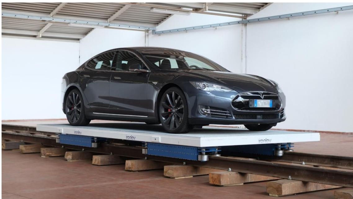
Figure 56.- Ironlev full scale platform on standard rail – loaded configuration. (Source: Ironbox)
