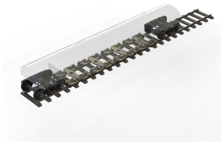
Figure 61.- Ironlev bogie coupled with standard bogie - overview. (Source: Ironbox)
