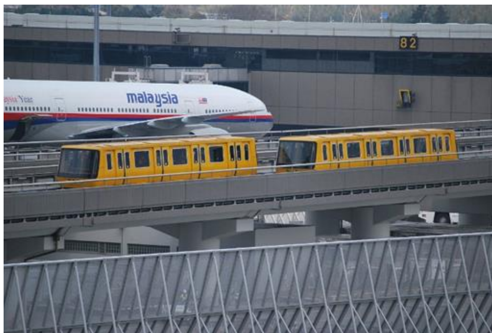
Figure 79.- Horizontal elevator using air-cushion technology in Japan (Source: https://en.wikipedia.org/wiki/Otis_Hovair ).
