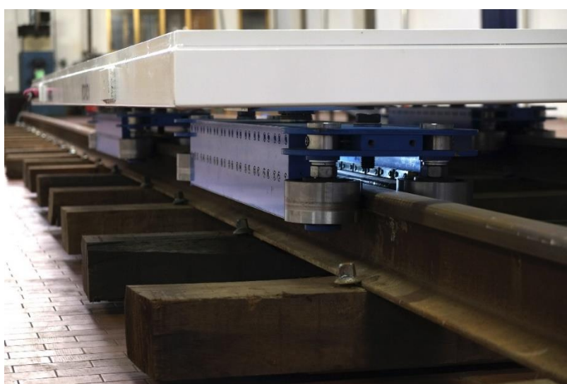
Figure 55.- Ironlev full scale platform on standard rail – side view. (Source: Ironbox)
