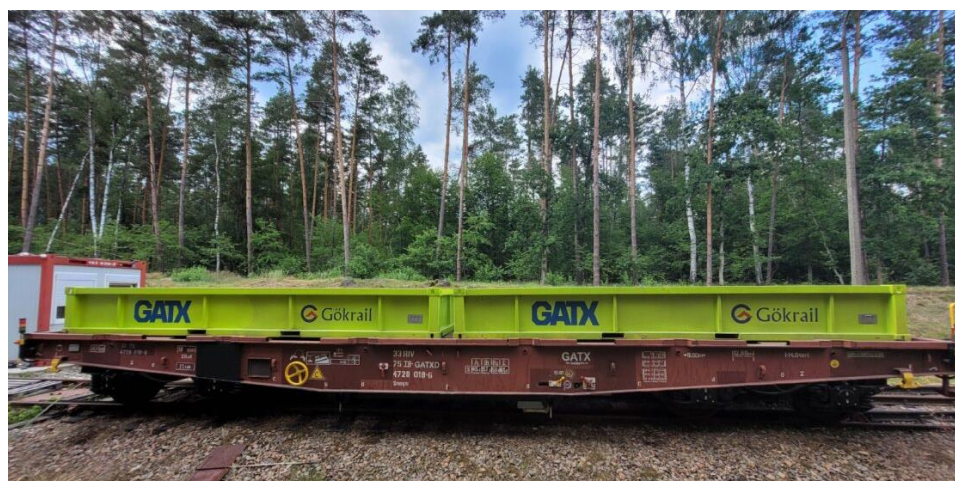
Figure 86.- The MagRail Booster with GATX platform. (Source: Nevomo)
